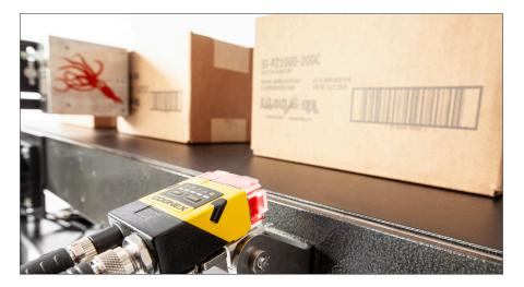
SquidCheck is integrated with a Cognex® reader and Squid Ink printer to ensure that codes are present, scannable, and accurate.
