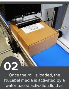
Once the roll is loaded, the NuLabel media is activated by a water-based activation fluid as the label is being fed onto the tamp pad. The label is then cut to length and applied with a tamp-blow application.
